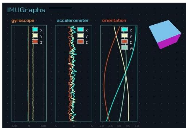
Figure 5 - Illustration of the data collection responsible for the spatial representation of the bracelet (cube) through the IMU.
