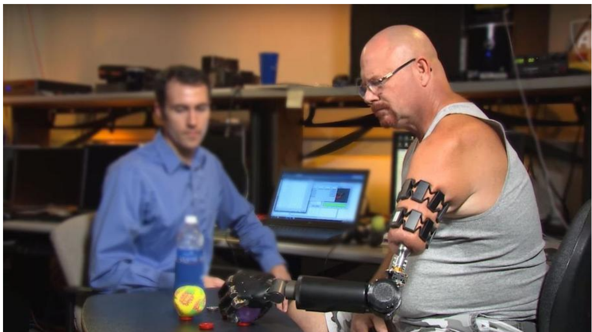
Figure 5 – Myo and the interaction with a mechanical arm
